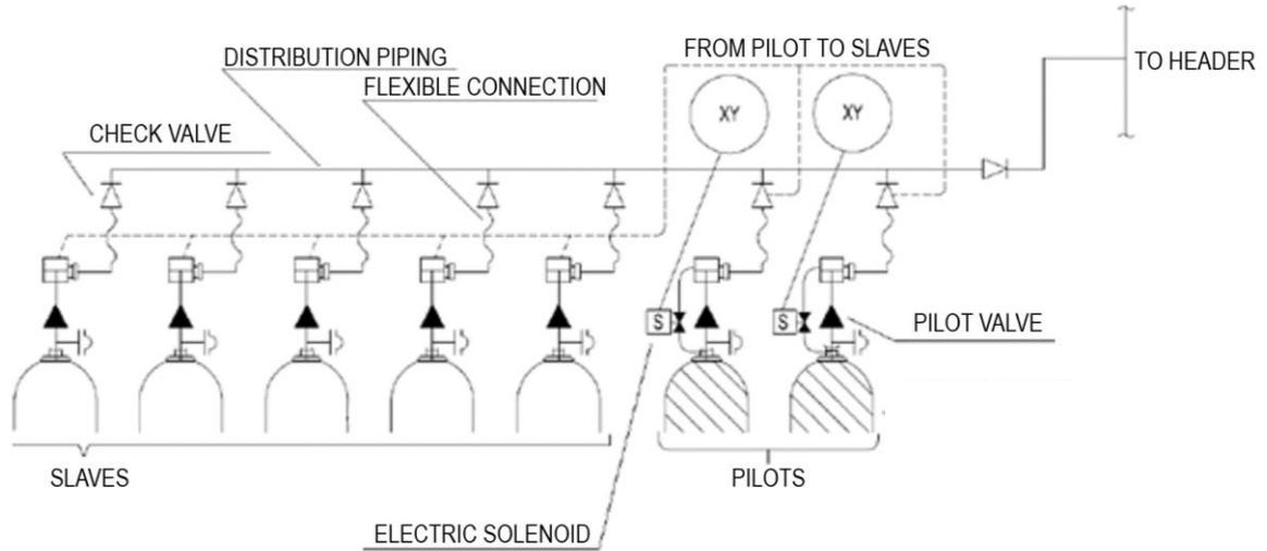
**7.2 Annex II – Logic for IG-541 fixed firefighting total flooding system**
